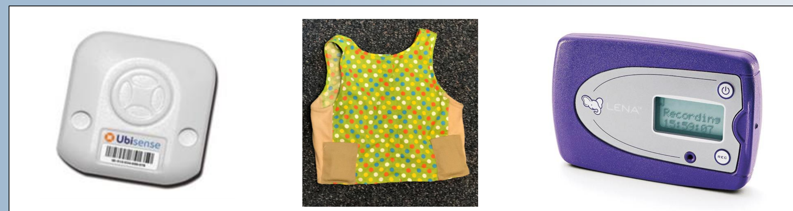
Figure 1: (from left) Ubisense tag, vest worn by children that holds LENA and Ubisense devices, LENA audio recorder
