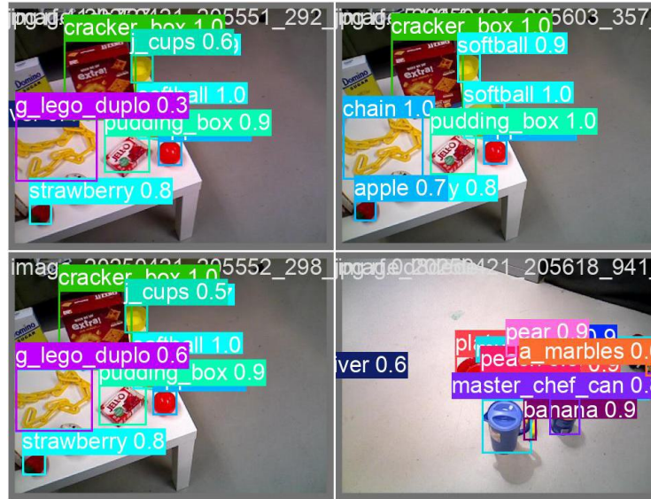
Fig. 4. Validation batch prediction demonstrating performance on cluttered scenes.
