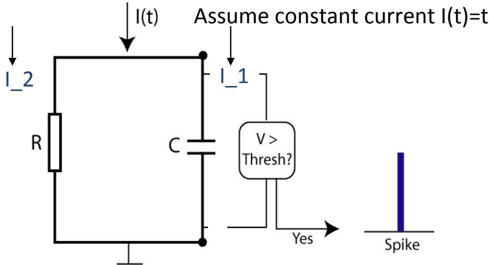
(1)  $C V = Q$  (C capacitance; V voltage; Q charge)
