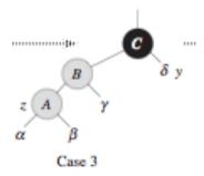
Main steps for case 3: The fix in this case includes both recoloring (between z.p and z.p.p) and rotation (between z.p and z.p.p):
