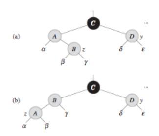
Here z (also labeled node A) is the inserted node; we denote the grandparent (node C) z.p.p, and the other child of the grandparent y (also labeled node D). We draw the subtrees of the nodes, and note that this could either happen at the initial stage of insert (in which case z's children are nil) or during a recursive step.
