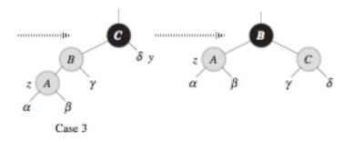
Following the recoloring and rotation, we have a valid Red Black tree. Note that after applying the fix for case 3 one time, we are done, because there is no longer a two Reds in a row violation; the Black height property is maintained; and the root is guaranteed to be Black.
