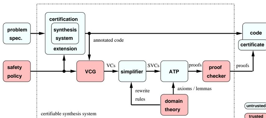
Figure 1: Certifiable program synthesis: System architecture
